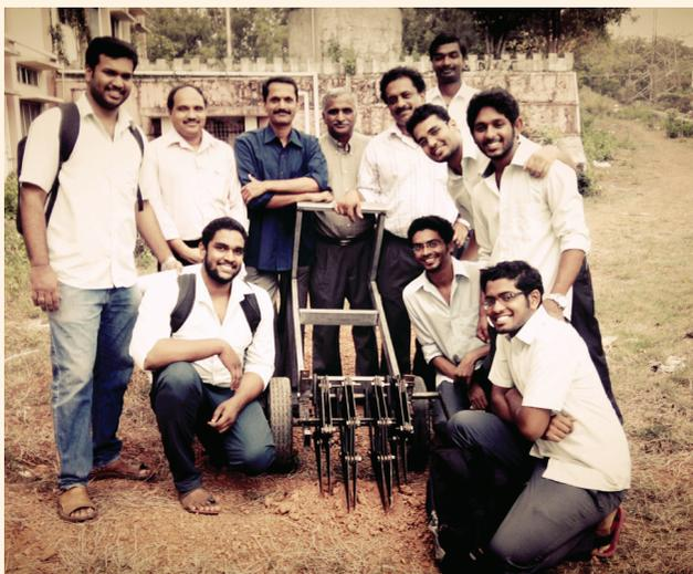
A team of students of School of Engineering, Cochin University of Science and Technology has developed a ploughing machine which is portable and maneuverable as a land mower and is proposed to be an alternative to manual plough-
